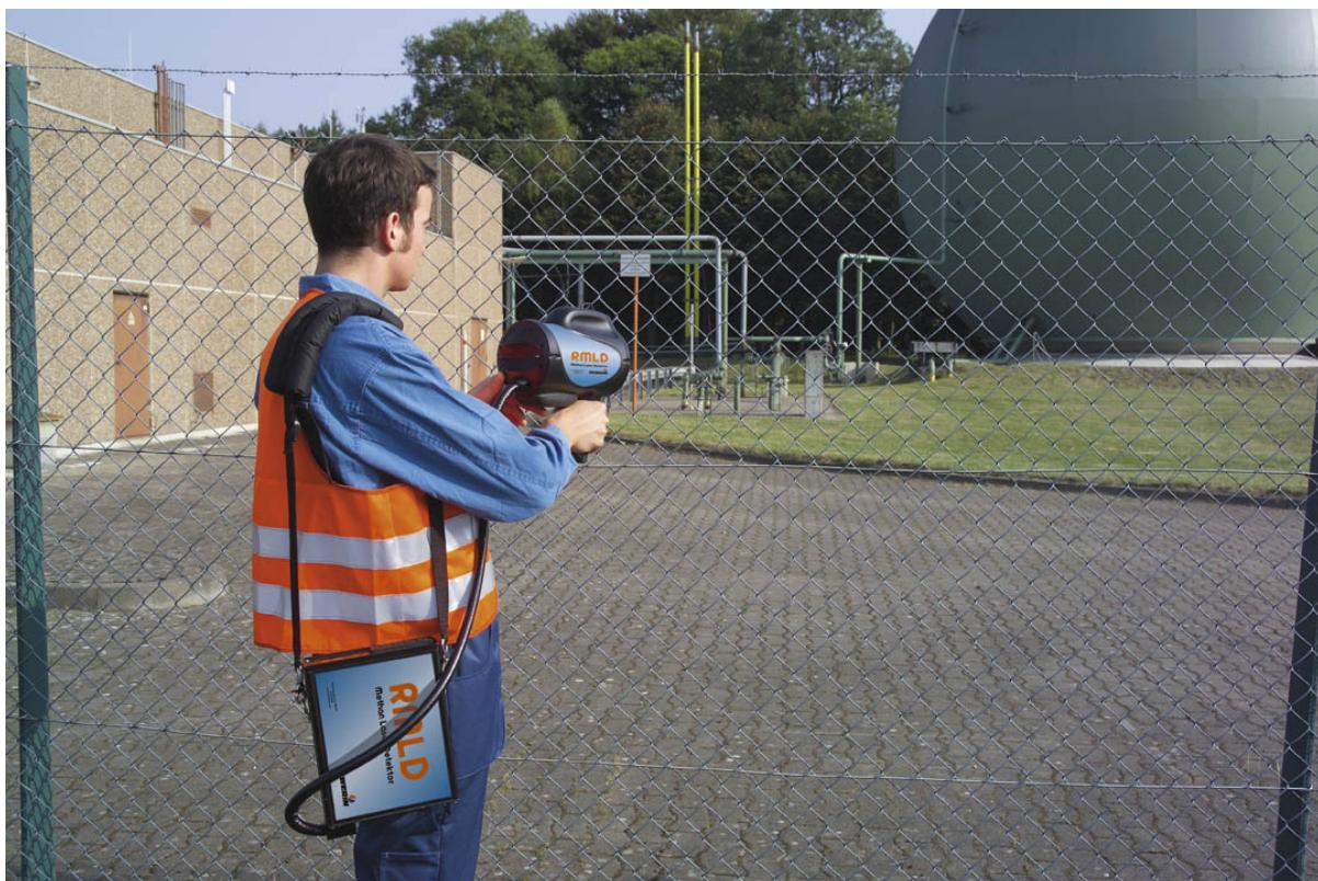
The Sewerin **RMLD** (Remote Methane Leak Detector) is the first instrument in a generation of laser leak detectors, allowing the user a completely new method of operation.
